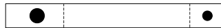
Design Condition 1 Wall pier with uniform thickness and ETABS-determined (variable length) edge members
