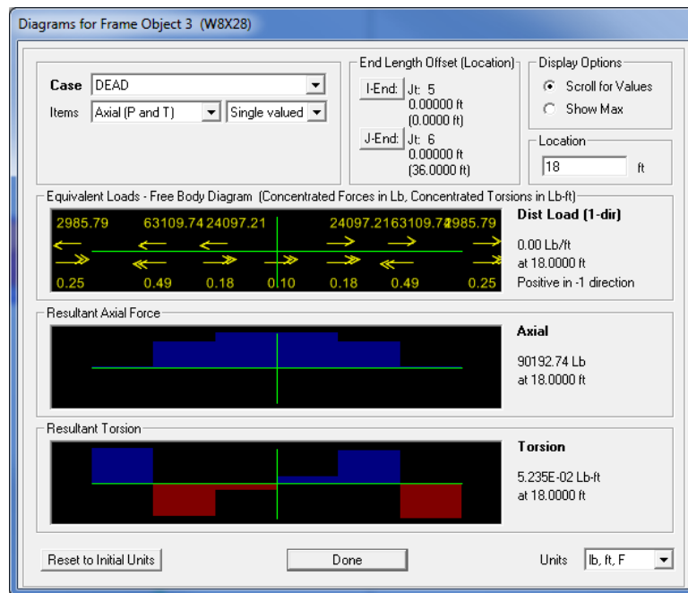
Figure 46 Force details obtained by right-clicking bottom chord of truss in the elevation view in Figure 45
