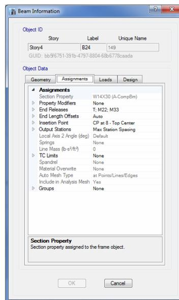
Note that the Design tab reports that the Design Procedure is Composite Beam. The program assigned this default design procedure to this frame object because (1) it lies in a horizontal plane, (2) the ends of the beam are pinned (that is, moment is released at each end of the beam), and (3) it is assigned a steel section that is either I-shaped or a channel.
