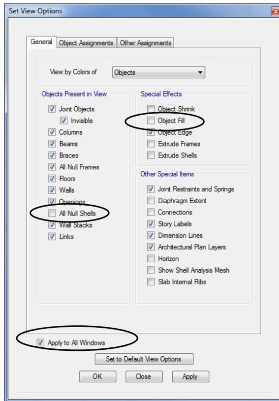
1. In the Objects Present in View area of the form, uncheck the *All Null Shells* check box.
