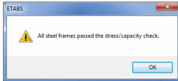
Note that members not passing at this stage is an indication of inadequate sections in the auto select list. The program would have used the largest section in the auto select list for both analysis and design, finding it inadequate. In that case, either add more sections to the auto select list or assign a larger section to the members that did not pass and continue with the design process. Click the **OK** button to close the form.
