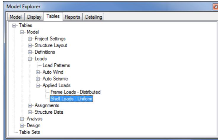
1. Right click on the Shell Loads - Uniform leaf and from the context sensitive menu select **Show Table**. The table shown in Figure 49 is displayed along the bottom of the program window.
