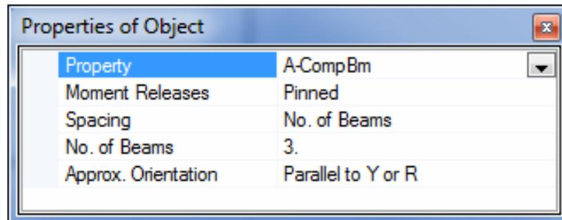
Make sure that the Property item is set to *A-CompBm*. If it is not, click once in the drop-down list opposite the Property item to activate it and then select *A-CompBm* from the resulting list. *A-CompBm* is a built-in auto select section list intended to be used for composite secondary beams. Review the sections included in the *A-CompBm* auto select list as follows: (1) click the **Define menu >**
