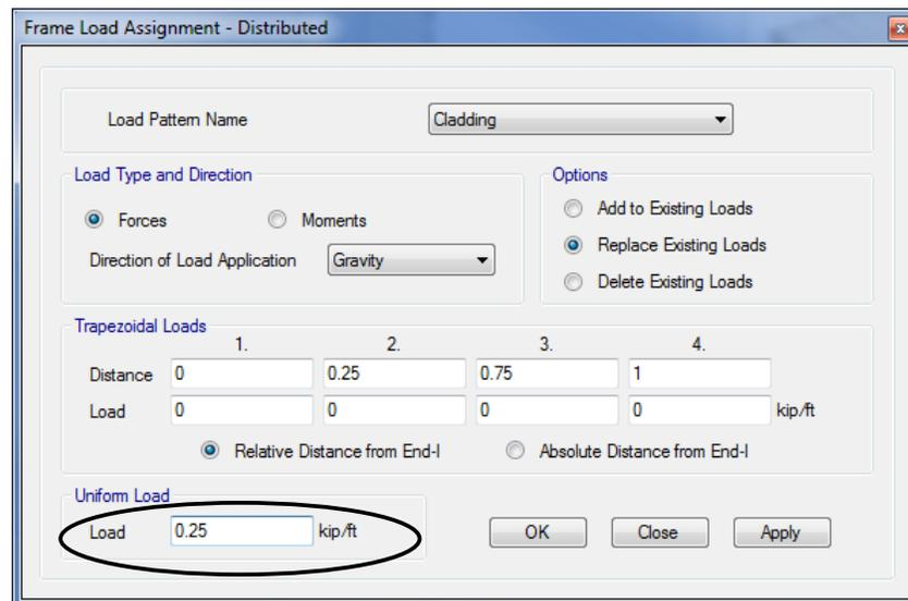
1. Verify that the units are set to kip/ft and then enter **0.25** in the Load edit box that is located in the Uniform Load area of the form.
