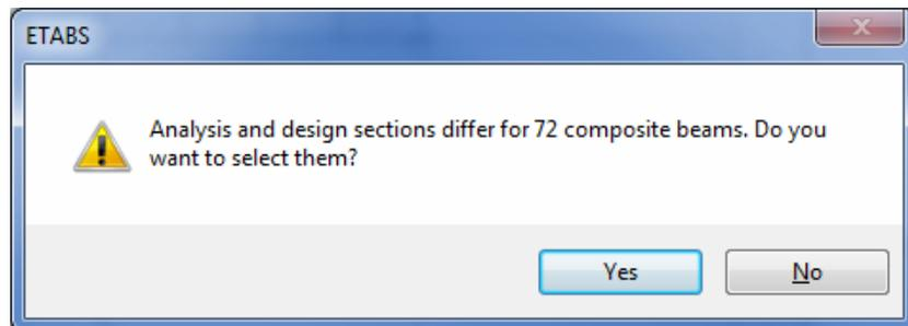
The goal is to repeat the analysis (Step 10) and design (Step 12) process until the analysis and design sections are all the same. Note that when the building is reanalyzed (i.e., Step 10 is repeated), ETABS will use the current design sections (i.e., those selected in Step 12) as new analysis sections for the next analysis run. Thus, in the next analysis of this example, the composite beams will be analyzed using W12X19 analysis sections.
