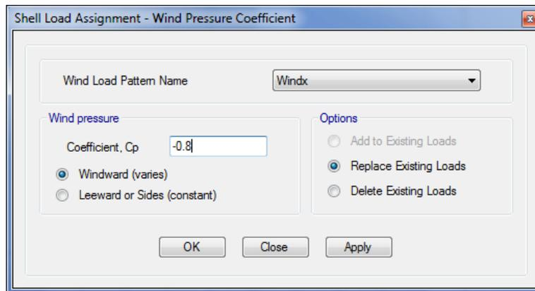
2. Click the **Apply** button to apply this load. Note that with the negative  $C_p$ , the load will act in the positive global X direction.
