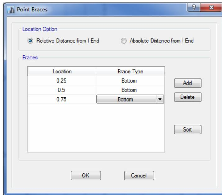
1. Verify that the *Relative Distance from I-End* option is selected - this allows ratios to be used for specifying the bracing locations.
