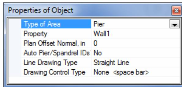
**Figure 5-18 Properties of Object Box for Walls**
