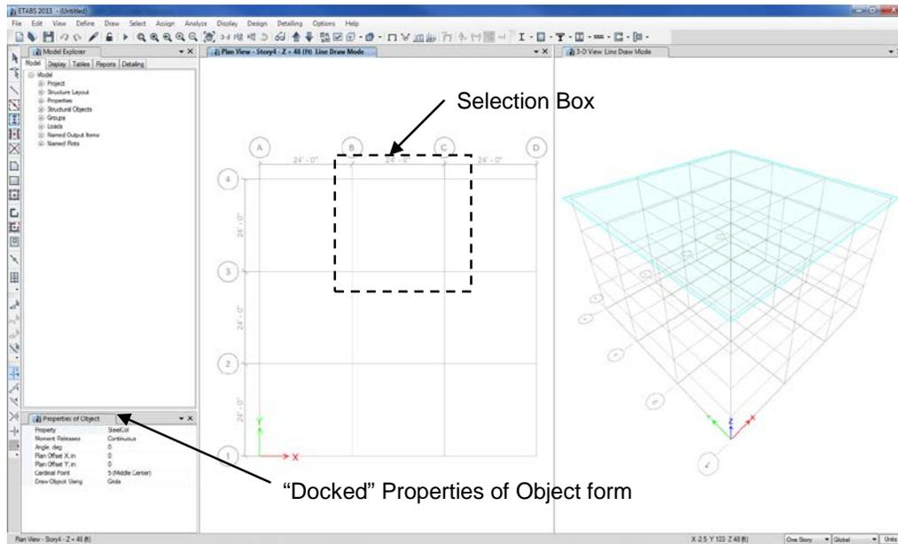
Figure 5-12 Drawing Column Objects in a Windowed Region
