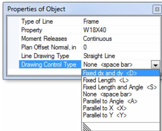
**Figure 5-14 Properties of Object Box for Frames**
