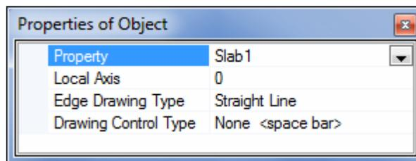
**Figure 5-16 Properties of Object Box for Shells**
