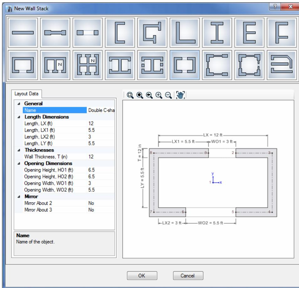
Figure 5-19 New Wall Stack form
