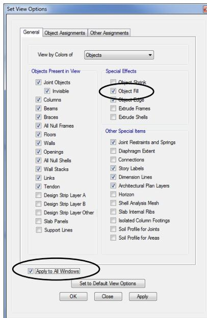
uncheck the Object Fill check box and the Apply to All Windows check box on the General tab, as shown in Figure 5-17. Click the **OK** button.
