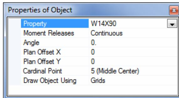
**Figure 5-11 Properties of Object Box for Columns**
