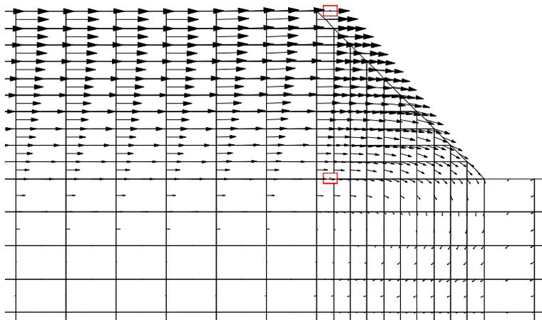
Figure 9-19 Displacement vectors
