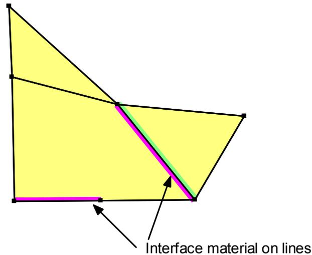
**Figure 3-11 Illustration of "interface elements" on geometry lines**
