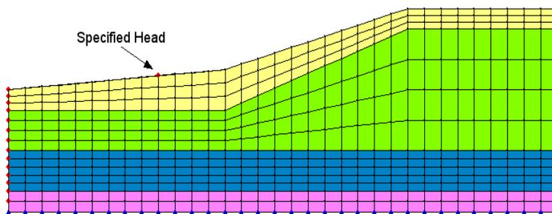
**Figure 2-15 Finite element model of stratigraphic section**
