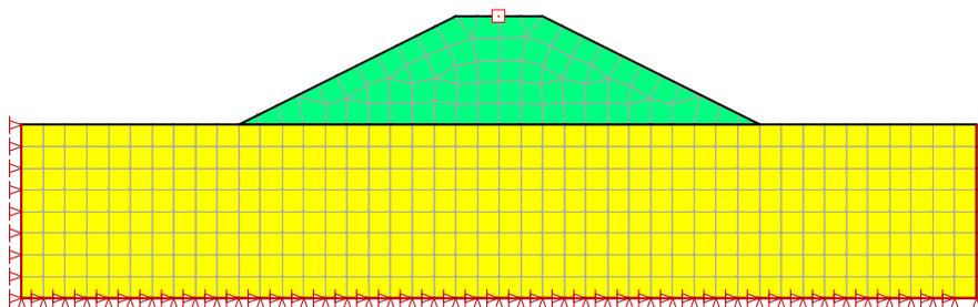
**Figure 6-8 Illustration of displacement boundary conditions**
