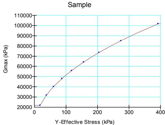
**Figure 4-7 A typical  $G_{\max}$  function for cohesive soil**
