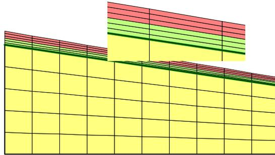
**Figure 3-21 Illustration of a surface layer mesh**
