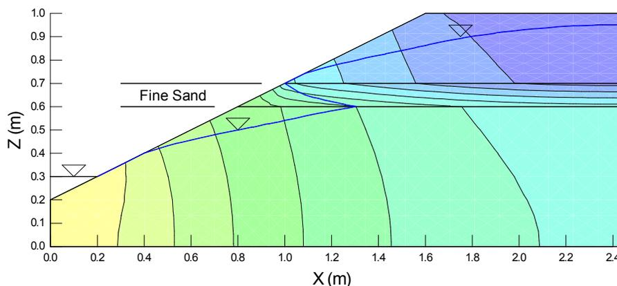
Figure 2-2 SEEP/W analysis of Rulon's laboratory model
