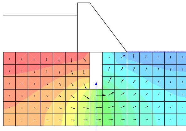
**Figure 2-17 Simple flow beneath a cutoff**
