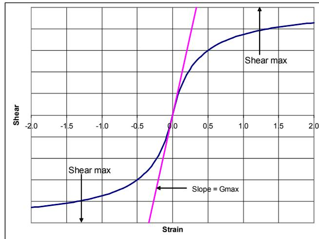
**Figure 4-3 Hyperbolic curve relative to  $\tau_{max}$  and  $G_{max}$**
