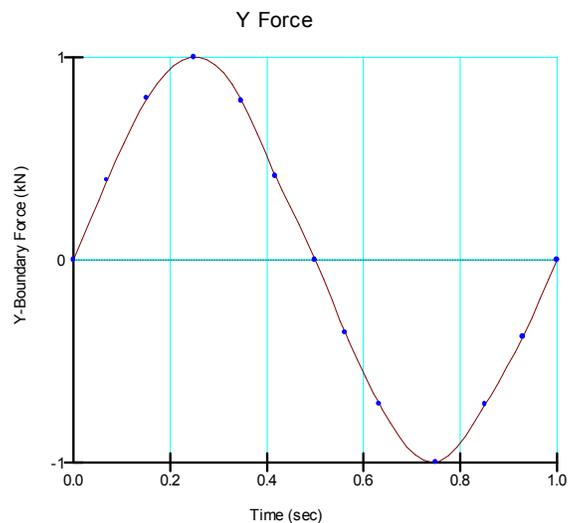
Figure 5-8 Example of a nodal force function
