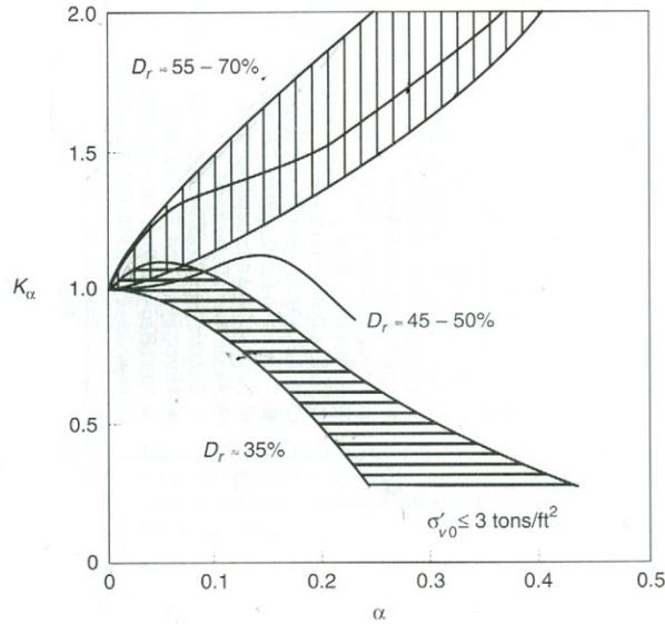
**Figure 9.32** Variation of correction factor,  $K_a$ , with initial shear/normal stress ratio. (After Seed and Harder, 1990. *H. Bolton Seed Memorial Symposium Proceedings*, Vol. 2, p. 364. Used by permission of BiTech Publishers, Ltd.)
