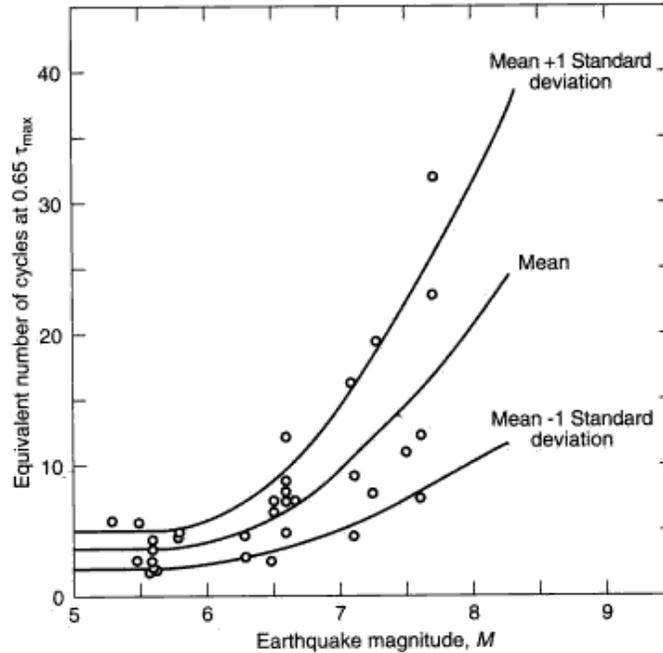
**Figure 4-11 Equivalent uniform cycles versus earthquake magnitudes**
