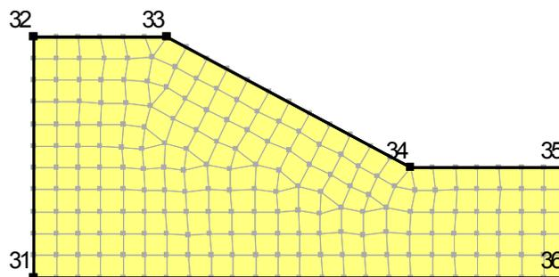
**Figure 3-17 Mixed quad and triangle unstructured mesh**
