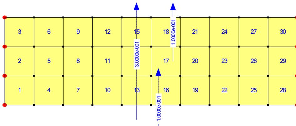
**Figure 2-16 Horizontal flow through three element section**
