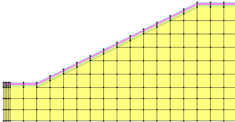
**Figure 3-25 Mesh showing angular surface slope breaks**
