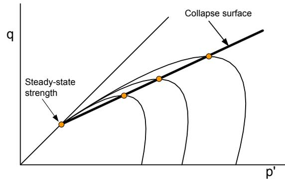
**Figure 4-26 Definition of collapse surface**
