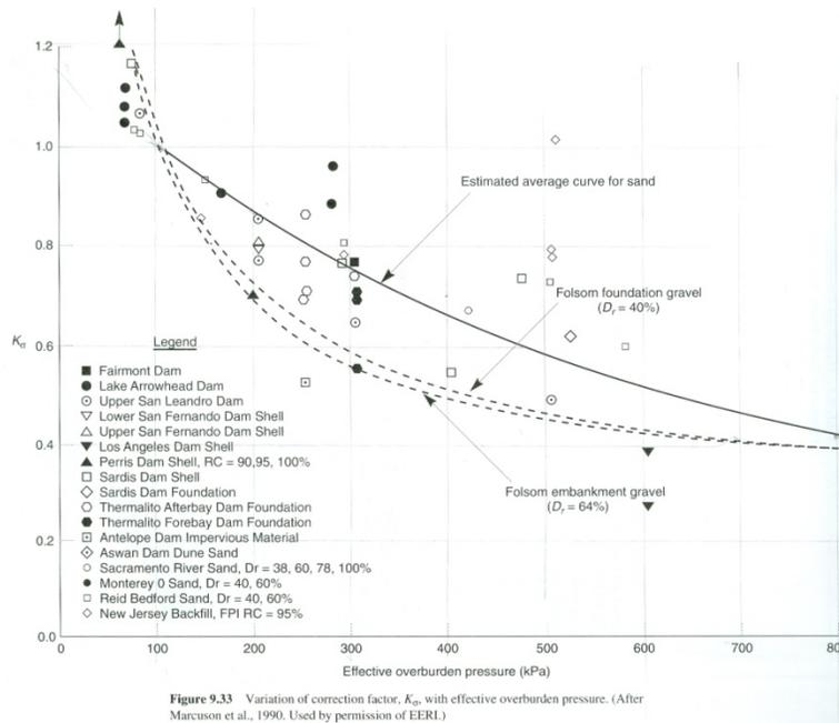
**Figure 4-17 Overburden correction factor  $K_s$**
