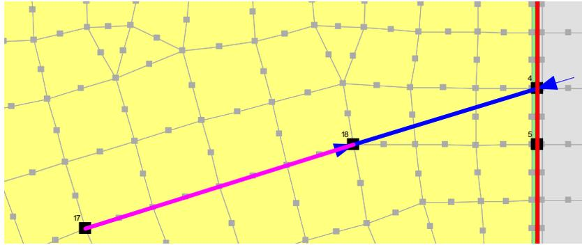
**Figure 3-9 Anchors on lines (line is partially meshed)**
