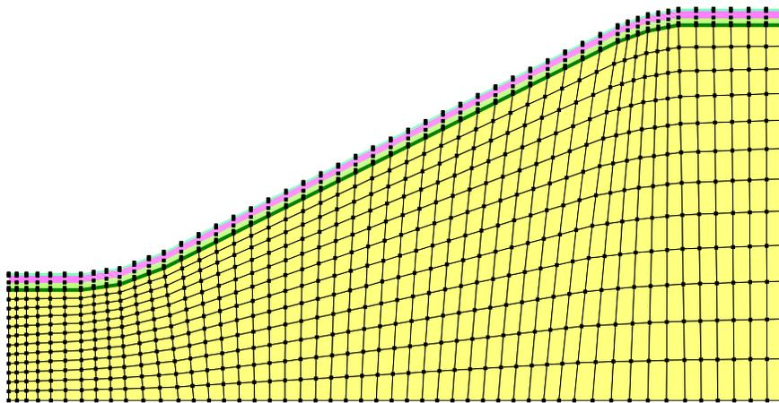
**Figure 3-24 Mesh showing rounded surface slope breaks**
