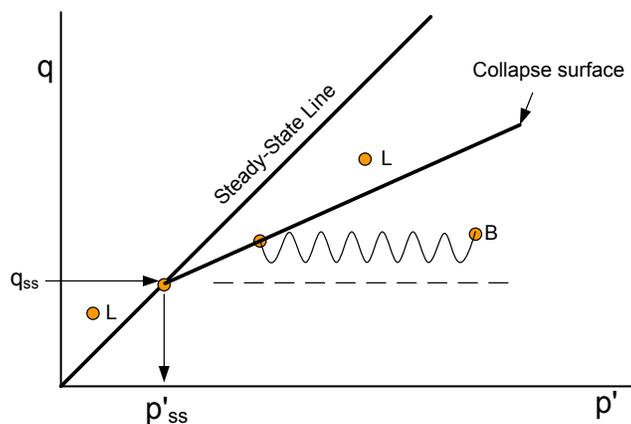
**Figure 4-29 Liquefiable zones in  $q$ - $p'$  space**
