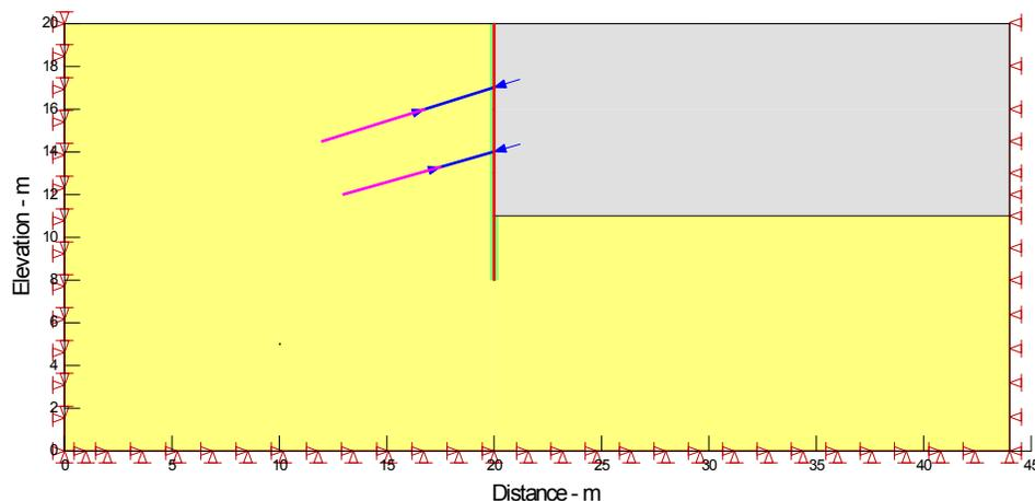
Figure 3-1 Fully defined geometry for soil excavation model
