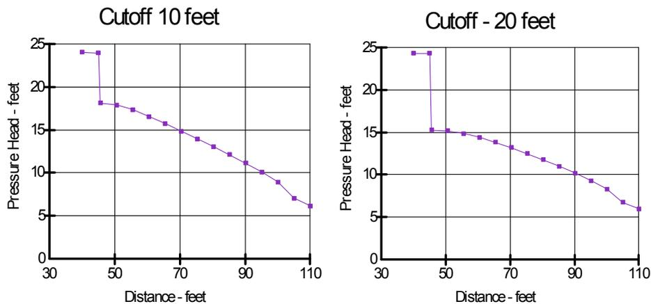
Figure 2-7 Uplift pressure distributions along base of structure
