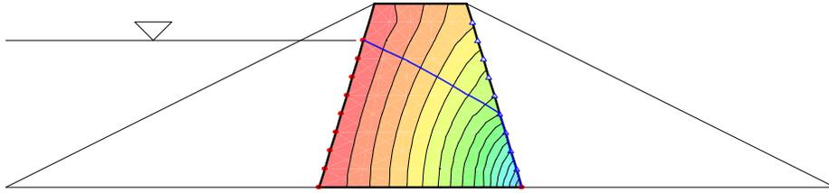
**Figure 3-36 Equipotential lines in core of dam**
