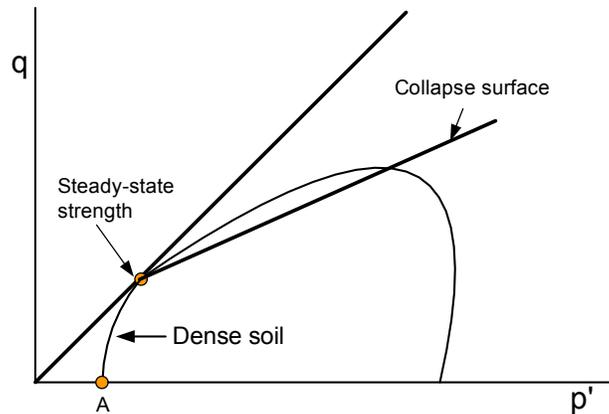
**Figure 1-7 Stress path for a dense dilative sand**
