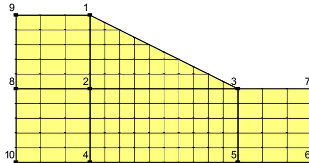
**Figure 3-16 Structured mesh**
