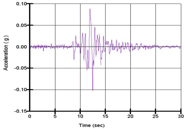
**Figure 5-3 An earthquake record with a baseline correction**
