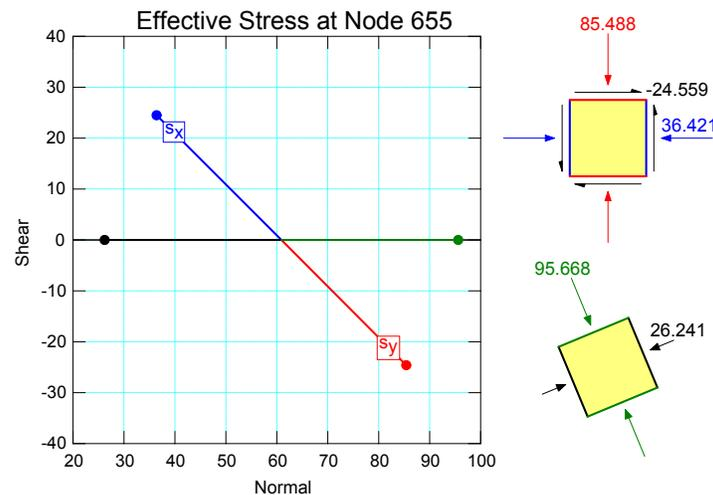
Figure 9-17 Mohr circle of stresses in an element
